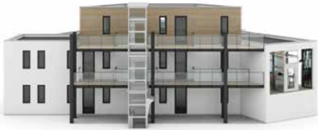
An outdoor lift preserves the space inside the building and of deck-access walkways.
